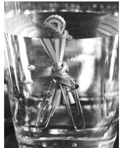
Hang paper clips on the rubber band until the diver floats correctly
